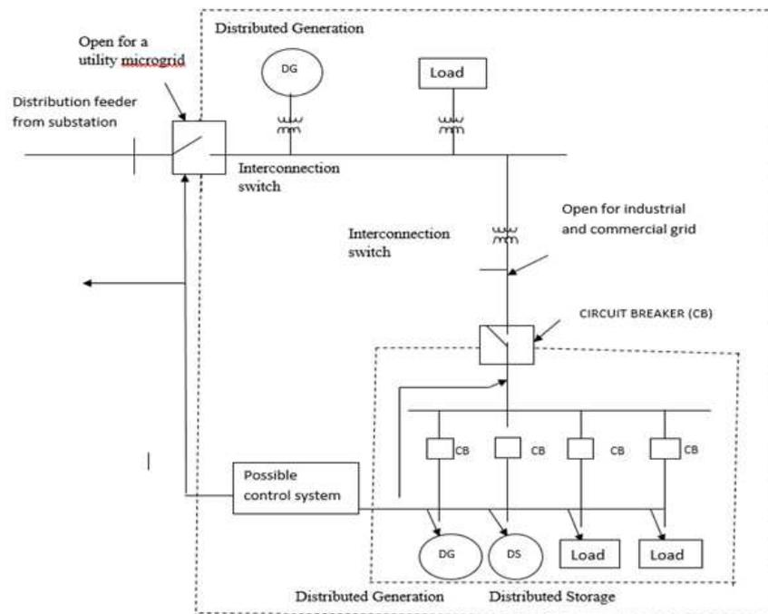
**Figure 2: Micro Grids and Components: [16].**
