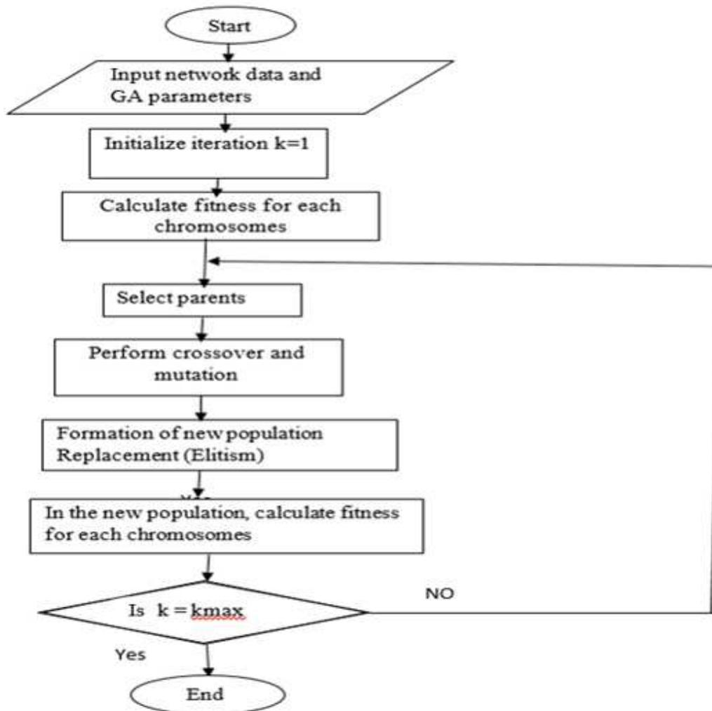
Figure 3.6: GAO Flowchart for Optimal DG Siting and Sizing. [36].
