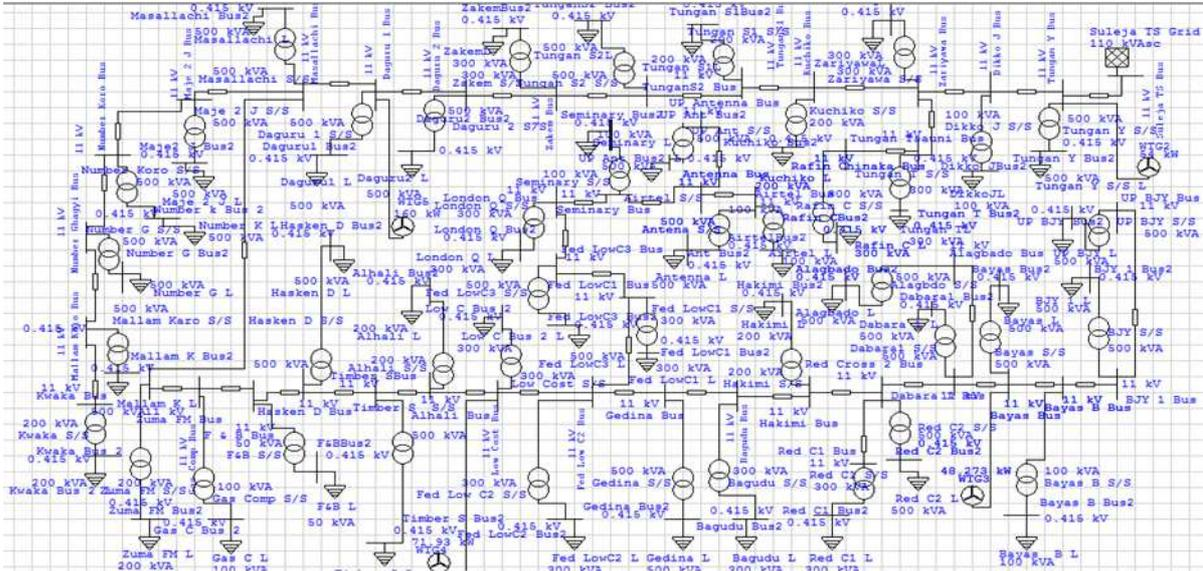
**Figure 3.8: ETAP Model of 11kV Dikko Feeder with DG Connected.**
