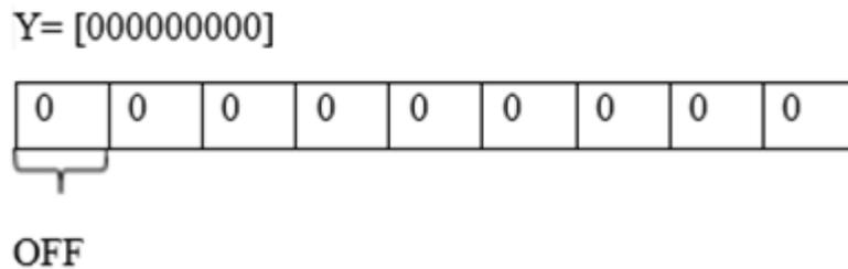
Figure 3.2: Illustrates Chromosome of a Generator Not Existing or Not Operating (Off).
