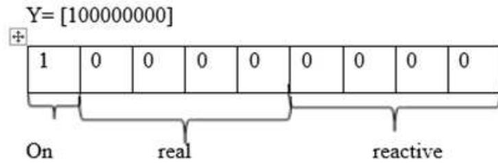
Figure 3.1: Illustrates Chromosome of a Generator Working at Minimum Capacity (on).
