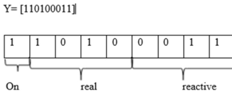
Figure 3.4: Illustrates Chromosome of a Generator Working at Active Power Capacity of 33.33% and Reactive Power Capacity of 80%,When Considering Fixed Weight of 8421.[45].
