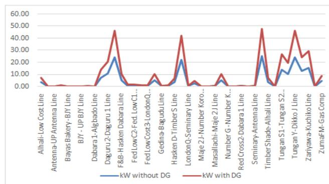
**Figure 4.3: Active Power Losses on Dikko Feeder With and Without DG.**
