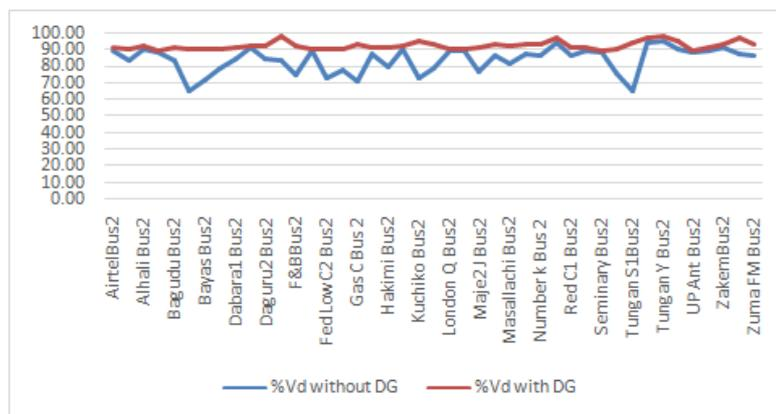
Figure 4.5: Voltage drops on Dikko Feeder With and Without DG.
