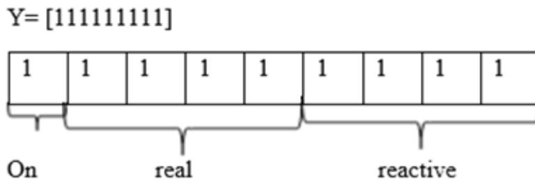
Figure 3.3: Illustrates Chromosome of a Generator Working at Full Capacity (On).
