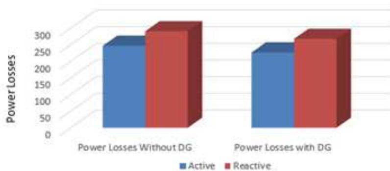
Figure 4.6: Bar Chart Representing Active and Reactive Power Losses.
