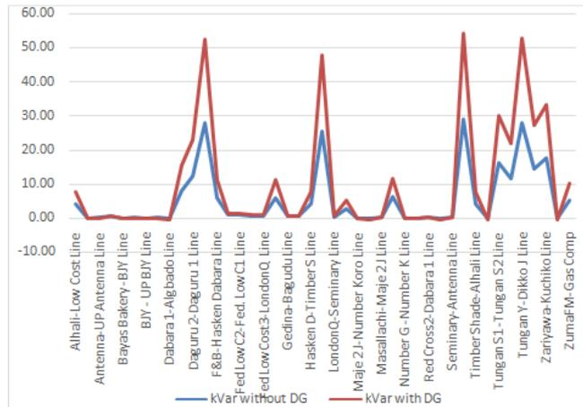
Figure 4.4: Reactive Power Losses on Dikko Feeder With and Without DG.
